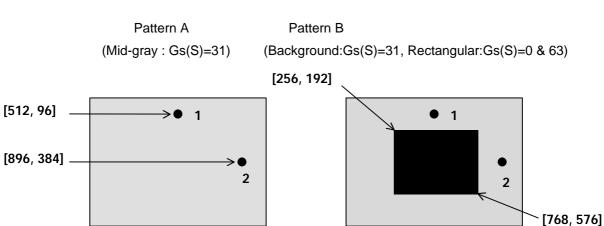
Vertical Crosstalk shall be measured at the location 1 and horizontal crosstalk shall be measured at the location 2.
